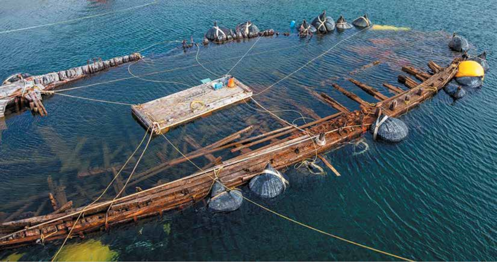
On a quiet evening, Maud can be seen with all the airbags attached around her hull.
