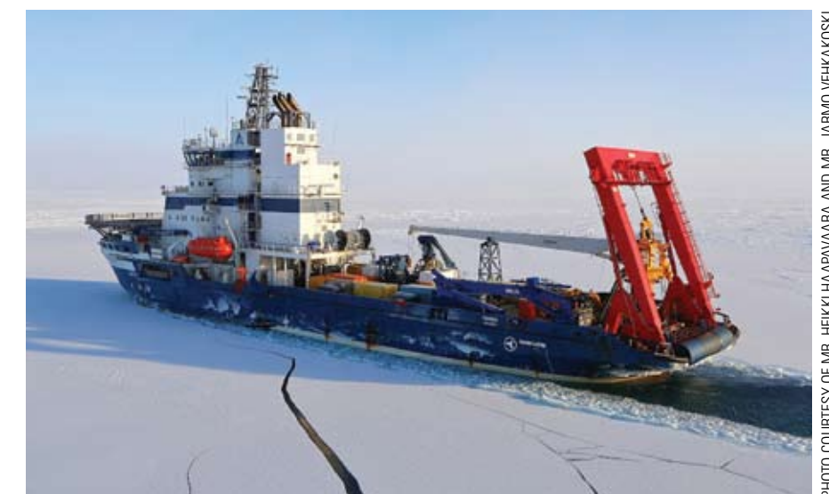
The Ice—Icebreakers require three traits most normal ships lack: a strengthened hull, an ice-clearing shape, and the power to push through sea ice.
